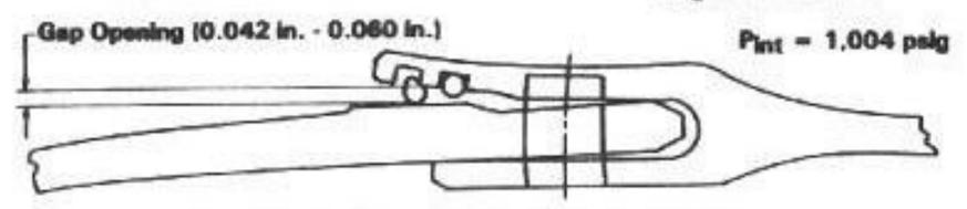
Preseurized Joint - Rotation Effect (exaggerated)
