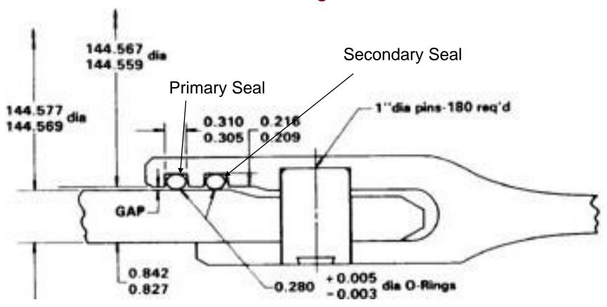
180 load carrying pins, Two O rings – Primary and Secondary seals Pressurization of the motor to 1004 psi (6.92 x 106 pascals) causes the gap dimension to increase 0.042 inches (1.07 mm).
